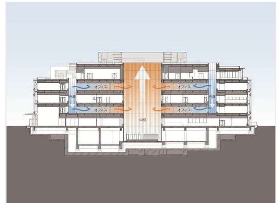
Natural ventilation system
