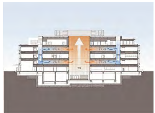
Natural ventilation system
