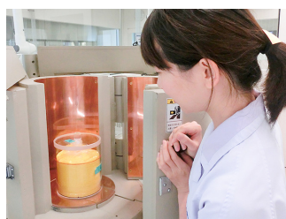
2. Placing a sample in a germanium semiconductor detector
