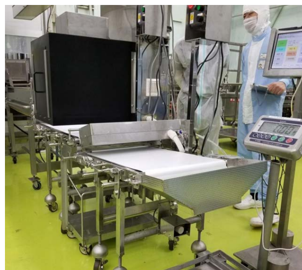
The world's first non-annotated machine learning ingredient inspection system installed at a manufacturing site
